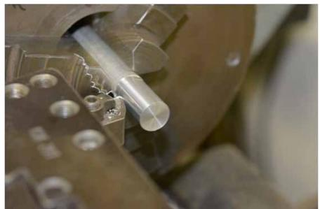
An insert was installed from both ends. The top side insert to accept the valve cover bolt and the bottom side insert to accept a .500 long metric set screw that would connect the new boss to the head (thanks to Ted Crum for the suggestion).
