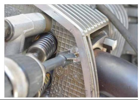
The head was drilled and tapped for a Heli-coil threaded insert and the insert was screwed in with Lock-tite.
